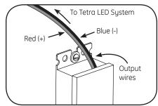
Connect the supply wire that is attached to the Tetra LED System to the red (+) and blue (-) output wires of the power supply as outlined in the "Electrical Connections" section of your LED system's Installation Instructions.
