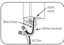
Connect the AC line to the black (line) and white (neutral) input wires of the power supply using 18-14 AWG (0.82-2.08 mm²) twist-on wire connectors.
