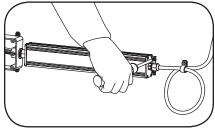
Mount Power Supply in a horizontal orientation with a minimum of one screw per mounting plate (two screws per power supply) with the base in contact with the mounting surface in accordance with the power supply spacing requirements described above.
