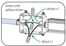
Connect the AC line to the black (line) and white (neutral) input wires of the power supply using 18-14 AWG (0.82-2.08 mm²) twist-on wire connectors. Properly ground (green wire with yellow stripe) power supply in accordance with National Electric Code (NEC) Article 600.
