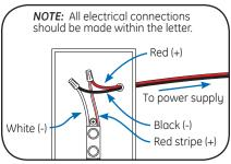
Connect the red stripe wire (+) of the LED to the red wire (+) of the power supply. Connect the white wire (-) of the LED to the black wire (-) of the power supply.
