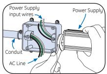
1 Run AC line through conduit and attach conduit to outdoor-rated/UL approved enclosure. Attach power supply to enclosure.
