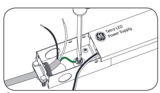
Connect AC line ground wire to Junction Box ground screw.
