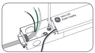
Mount and secure Junction Box and Tetra Power Supply using #6 or #8 screws and star-type lock washers in both holes.
