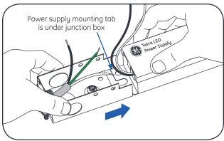
**3B** For all other power supplies: Slide junction box onto AC input end of power supply and align mounting holes. Ensure power supply mounting tab is under the junction
