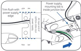
3A For GEPS24-100U-GLX only: On the AC input end of power supply, trim or grind sides of mounting tab flush with power supply. Then slide junction box onto AC input end of power supply and align mounting holes. Ensure power supply mounting tab is inside the junction box.
