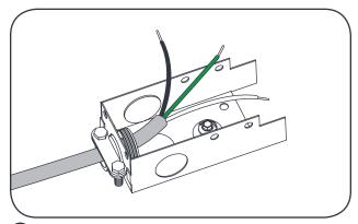
2 Select a wire entry knock out location and carefully remove metal plug. Install wire box fitting and supply wire and secure in place.
