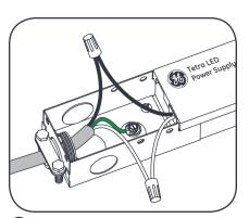
Connect Tetra Power Supply to AC line per instructions enclosed with the power supply.
