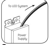
Run a wire from the Power Supply and connect to the first LED module on the strip.
