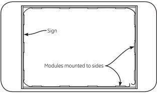
1 Determine location of where LED modules will be mounted based on sign dimensions (see chart). If mounting on bottom of sign, the use of a riser will be needed (minimum 1/8 in. distance between bottom surface and module).
