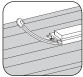
Cap all exposed wires with appropriate end caps or apply electric grade (non-conductive) silicone for additional weather protection.
