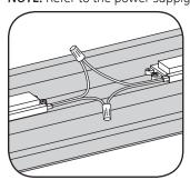
1 Connect modules using twist-on wire connectors or in-line (IDC) connectors. Join white wires together and red striped wires together.
