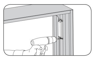
4 Use rivets, screws, or silicone to secure each module within the sign. Use #6 (M3) or #8 (M4) screws, 1/8-inch (3.2 mm) rivets, or silicone.
