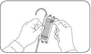
Peel off backing to expose adhesive tape and stick LED modules into place.
