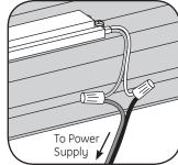
Connect the red stripe wire (+) of the LED system to the red wire (+) of the power supply. Connect the white wire (-) of the LED system to the black or blue wire (-) of the power supply.
