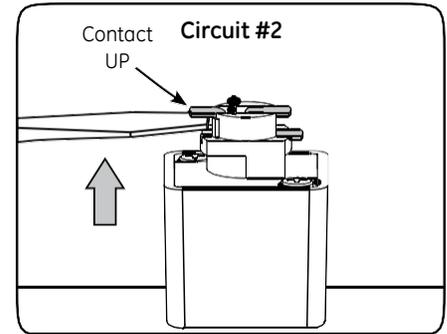
**Two-circuit systems:** Lift the lower contact to the up position with a narrow blade screw driver.
