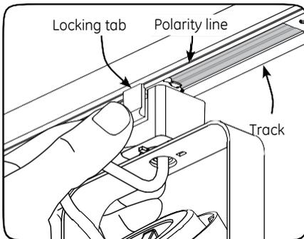
**1** Hold the adapter below the track with your thumb on the locking tab. Make sure the locking tab is positioned directly below the polarity line. Push adapter into track.
