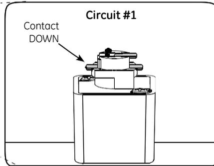
**One-circuit systems:** No adjustment is required. Contact is in the down position.
