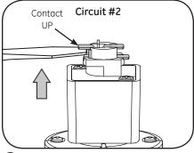
For two-circuit installation, lift the lower contact to the up position with a narrow blade screw driver.
