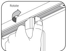
2 Rotate adapter 90 degrees clockwise, making sure the polarity lines match between the track and the fixture adapter.
