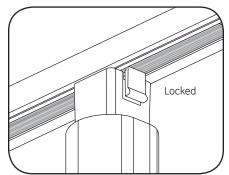
Release the locking tab and the fixture should snap into position.
