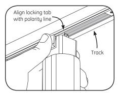
Hold the adapter below the track with your thumb on the locking tab. Make sure the locking tab is positioned directly below the polarity line. Push adapter into track.
